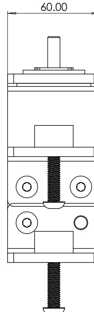
BOTTOM CLAMP CAN BE FITTED TO FOUR DIFFERENT POSITIONS TO COVER THE FULL RANGE OF DESK THICKNESS
